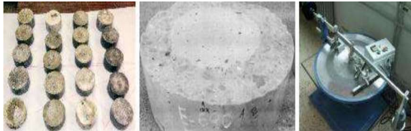
Fig.-7: Samples of Concretes Used in the Abrasion Test (Laboratory Abrasion Circle LKI-3)
